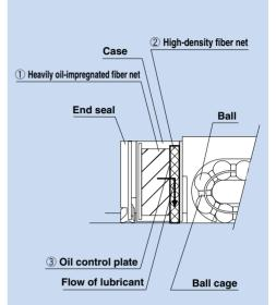
The structure of the QZ Lubricator consists of three major components:
