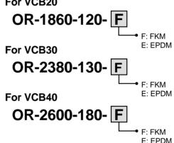
If external leakage occurs after replacing the coil, replace the above seals.
