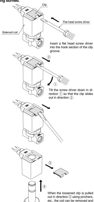
After replacing the coil, the clip is reinstalled by pushing it back in the direction opposite to its removal.
