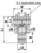
Applicable Tube: Metric Size, Connection Thread: M, R, Rc
