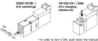
In order to turn it ON, push down the manual override button in the direction the arrow (→) indicates until it stops (approx. 0.5 mm), and release it to turn it OFF.
