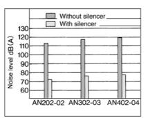
AN103 to 403 Condition: 0.5MPa at supply pressure of solenoid valve
