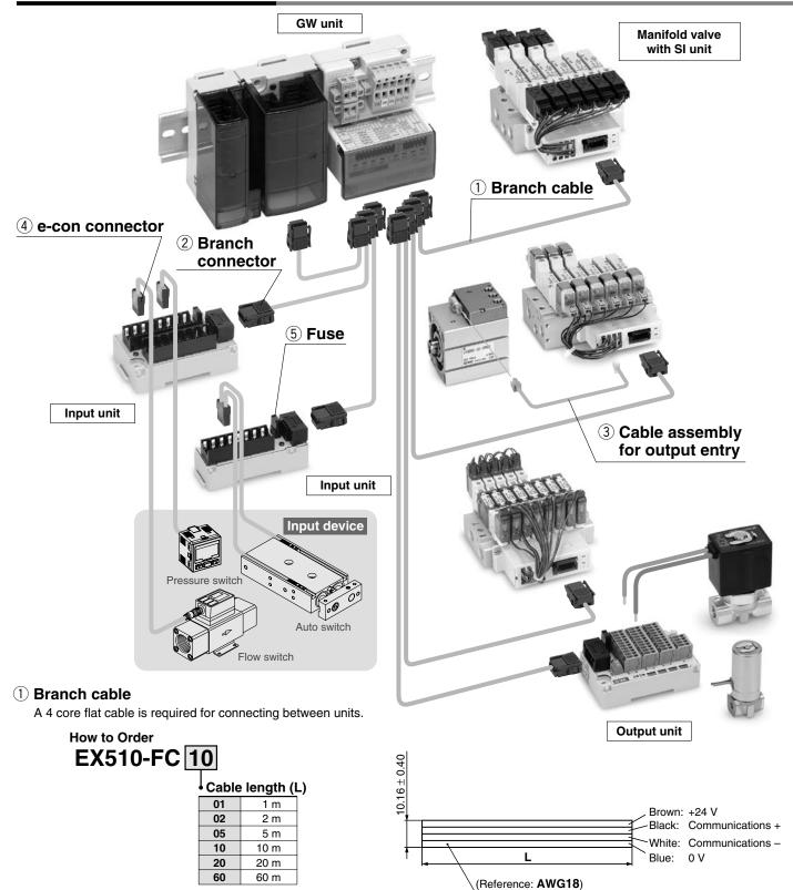
$<sup>^{\</sup>star}$  The maximum length of a branch cable for the EX510 series should be 20 metres or less.
