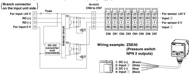
• EX510-DXP1 ··· Input unit for PNP (1 connector, 2-input type)
