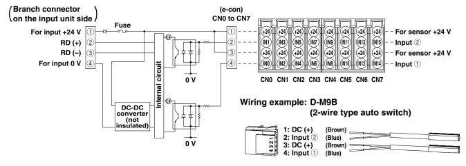
• EX510-DXN1 ··· Input unit for NPN (1 connector, 2-input type)
