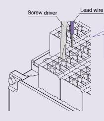
Torque control and crimping work is unnecessary.
