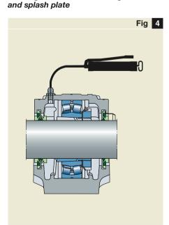
where the grease is applied, so that grease can only exit at the opposite side of the housing. For this purpose a set comprising a V-ring and a splash plate, which covers a sector of more than  $180^{\circ}$  ( $\rightarrow$  fig 4), can be supplied. This V-ring and splash plate set is designated by the prefix ASNA followed by the housing size identification and
