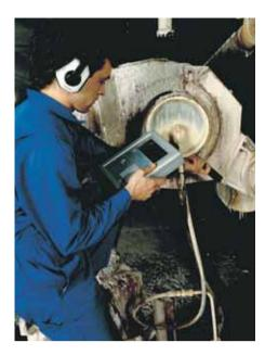
Recording vibration values using an SKF Microlog® data collection unit
