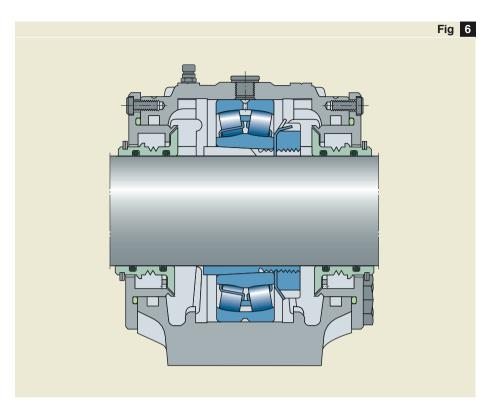
Housing for oil lubrication
