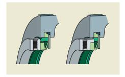
Recommended dimensions for support rings for V-ring seals
