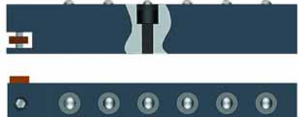
tee block secured by socket screw
