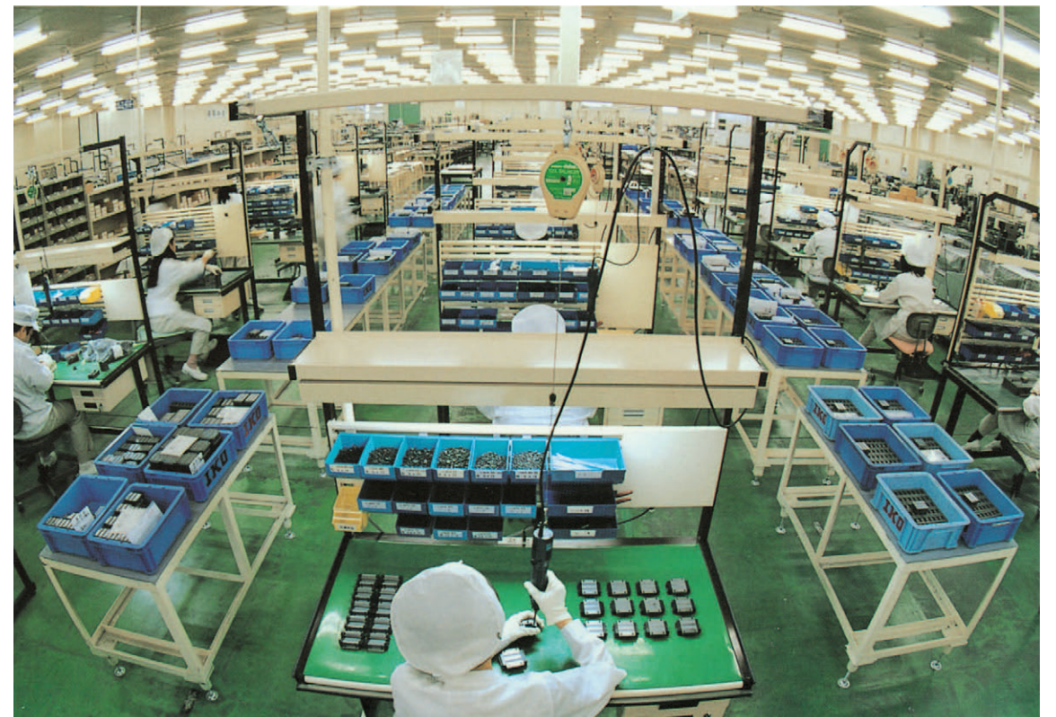
Assembling process in a clean room
