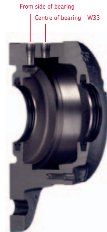
Pre-drilled holes enable relubrication from the side of the bearing or through the W33 groove.
