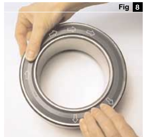
Inserting the retaining ring in the outer ring
